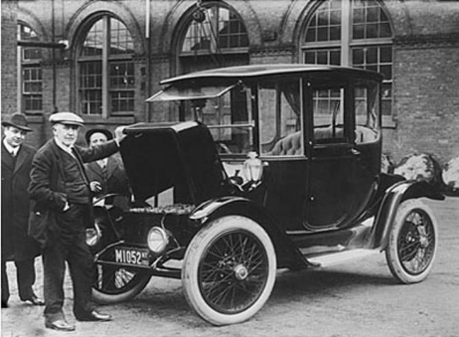
Thomas Edison inspects electric car in 1914. He and Henry Ford had planned to use Edison's nickel iron battery to power clean, efficient, affordable cars for the masses that would be recharged by home wind turbines, according to author Edwin Black in 'Internal Combustion'.
