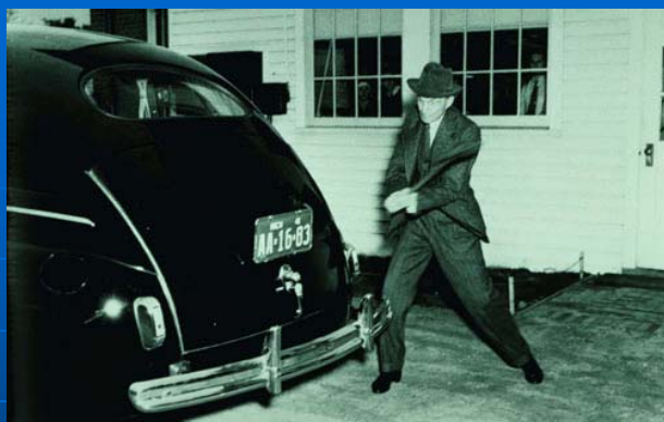
Henry Ford showed the strength of his soybean plastic car by hitting with an axe.
