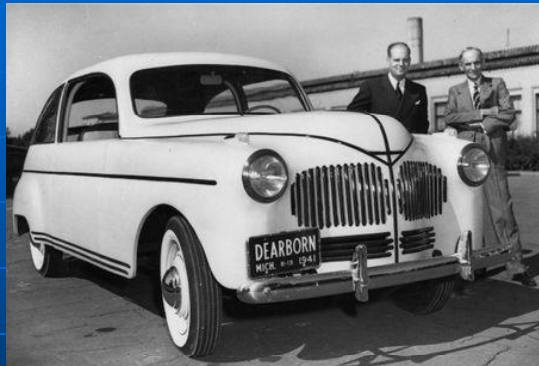
Henry Ford and Robert Boyer with the 1941 Ford made from soybeans. http://blog.hemmings.com/wp-content/uploads/2007/01/plasticford_resized.jpg
