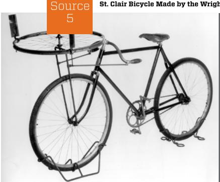
Years of methodical research led to the Wright brothers' first flight. This unusual bicycle measured air pressure. Riding the cycle caused the airfoils to spin the horizontal wheel. The bicycle's imprecise measurements led the Wrights to design and build a wind tunnel instead. Although the Wrights built this St. Clair, it is not the actual bike used in their experiments.
