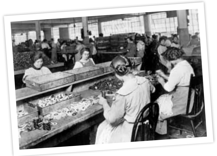
Women Workers Assembling Magnetos at Ford Highland Park Plant, circa 1913 ID# THF23810
