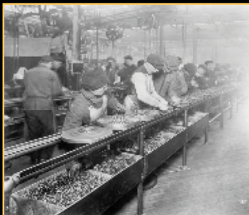
Applying magnets on Model T flywheels 1913
