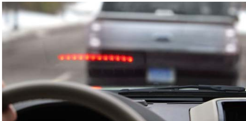
Visual warnings from Ford's Collision Warning with Brake Support technology
