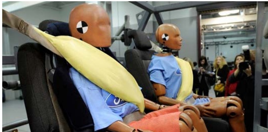
Inflatable safety belt technology
