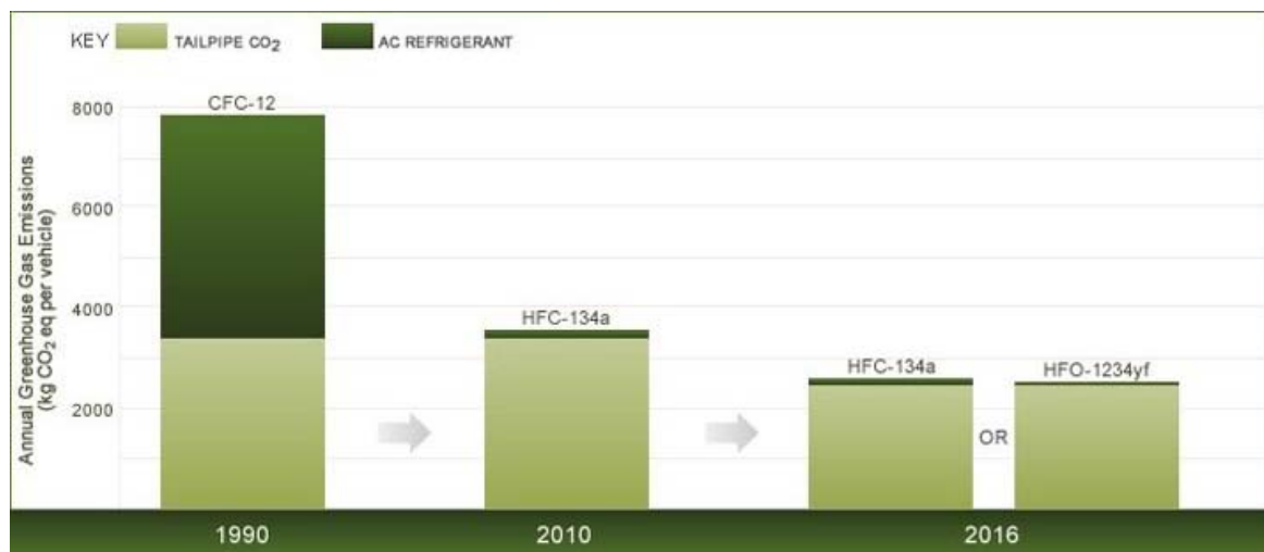
Figure 1: Annual in-use greenhouse gas (GHG) emissions from typical AC-equipped cars in the U.S in 1990, 2010 and 2016 using either CFC-12 (in 1990, left-hand bar), HFC-134a (2010 and 2016, middle bars), or HFO-1234yf (right-hand bar) refrigerants.
