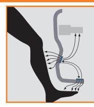
The detection of the leg motion breaks a miniature electrical field, alerting the system to respond. The effect of the leg movement is similar to motion technology employed by today's video games
