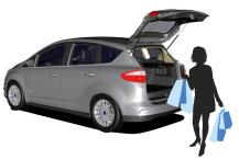
Belongings can be easily loaded into the cargo area. The height of the liftgate can be programmed to the customer's needs, either higher or lower
