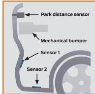
The motion sensors are located in two places in the bumper. One sensor detects the shin and the other detects the leg motion
