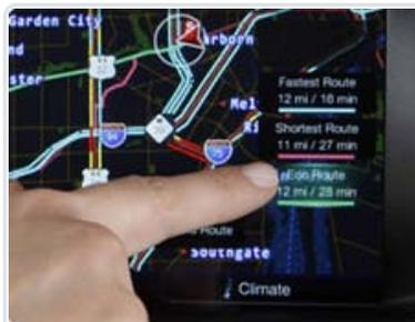
MyFord™ map-based navigation offers an Eco-Route option, which instantly calculates the most fuel-efficient route for the driver.
