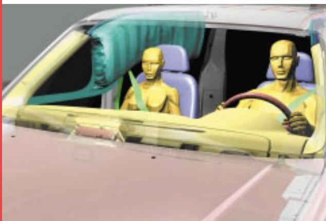
measure how fast the vehicle's lean angle is changing to determine if the vehicle is headed for a rollover. If a rollover situation is detected, the side curtain air bags are deployed, helping reduce injuries to passengers and keeping them inside the vehicle.
