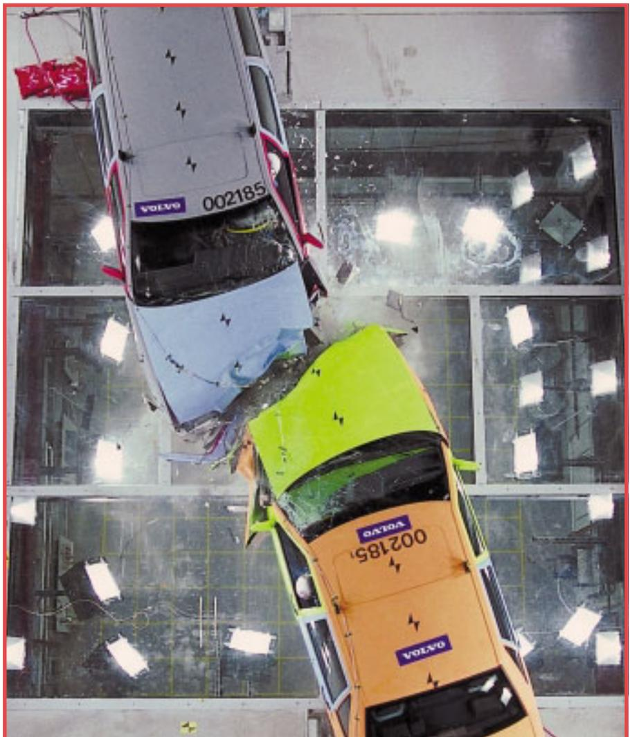
At Volvo Car's Safety Center in Gothenburg, Sweden, safety experts can reproduce full-scale collisions between a car and another car, a truck or a bus, at every conceivable angle under controlled conditions. The Center, used by Volvo and other Ford brands, provides data valuable in designing vehicles to perform well in the variety of accidents encountered in real-world driving.
