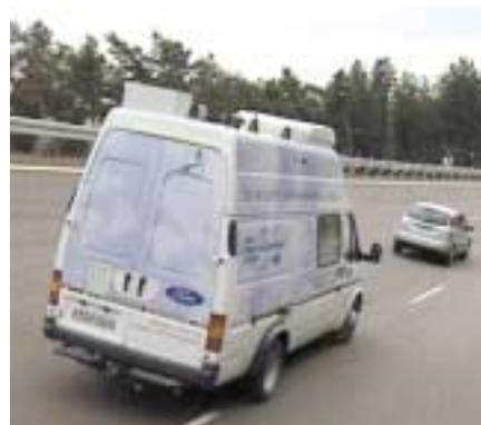
*The Ford Mobile Laboratory is equipped to collect emissions data from moving objects. Here it samples exhaust from a diesel test vehicle on a high-speed track.*
