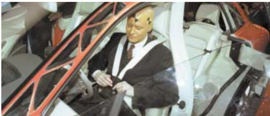
*“Clive,” the crash test dummy, buckles up with a four-point safety harness in the Volvo Safety Concept Car, designed and built jointly by Ford and Volvo, that also features a see-through A-pillar. 🚗*
