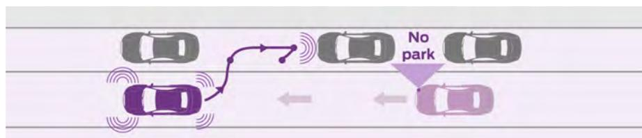
Active Park Assist uses ultrasonic sensors, while the driver is slowly driving near parking spots, to measure the space available. When a suitable parking space is found, Active Park Assist can steer the car into the parking space while the driver controls the shifting, accelerator and brake. Active Park Assist is available on certain Ford and Lincoln vehicles in North America, Europe and China.
