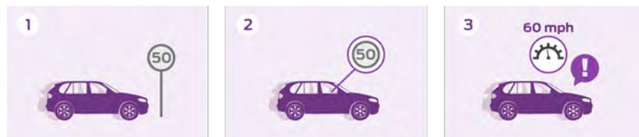
Traffic Sign Recognition uses a forward-facing camera that recognizes speed limit signs that use the standards of the Vienna Convention on Road Signs and Signals. The identified speed is then indicated in the instrument cluster to inform the driver of the speed limit. Traffic Sign Recognition will also warn the driver if the speed limit is exceeded. This feature is available in Europe.
