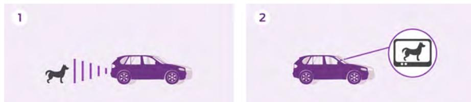
Our Rear View Camera transmits an image of what is behind the vehicle when the driver shifts to reverse. Rear View Camera is available on every Ford and Lincoln vehicle in North America and several Ford vehicles in Europe.
