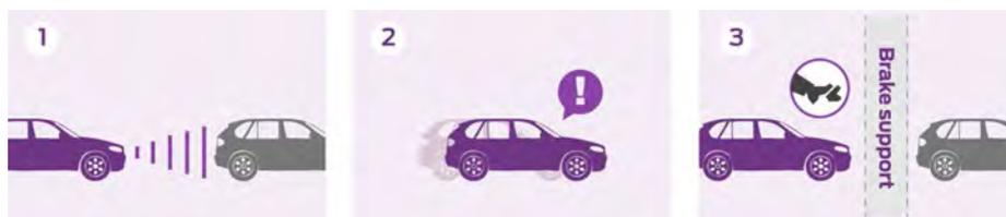
Ford's Forward Collision Warning with Brake Support technology uses the same radar module as Adaptive Cruise Control to detect range and speed. Forward Collision Warning
