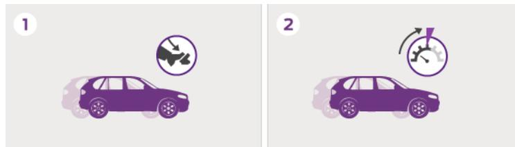
**Adjustable Speed Limiter Device (ASLD)** allows the driver to set a speed limit that cannot be exceeded by standard gas pedal operation. The driver can override the limit, however, by pressing the accelerator pedal beyond normal usage limits (>90 percent pedal travel). ASLD is offered on select Ford Motor Company vehicles in Europe and China.
