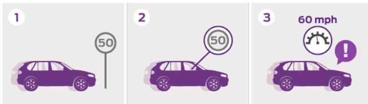
With **Traffic Sign Recognition**, a front camera recognizes speed signs that use the standards of the Vienna Convention on Road Signs and Signals. The identified speed is then indicated in the instrument cluster to inform the driver of the speed limit. If activated, the cluster will also warn the driver if the speed limit is exceeded. Traffic Sign Recognition is available in Europe.
