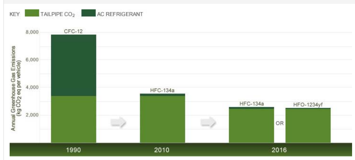
Figure 1: Annual In-Use Greenhouse Gas (GHG) Emissions From Typical AC-Equipped Cars in the U.S in 1990, 2010 and 2016 Using Either CFC-12 (in 1990, Left-Hand Bar), HFC-134a (2010 and 2016, Middle Bars), or HFO-1234yf (Right-Hand Bar) Refrigerants.
