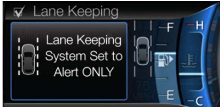
Our Lane Keeping System uses a small, forward-facing camera behind the inside rearview mirror to “look” down the road, monitor lane lines to determine that the vehicle is on course.
