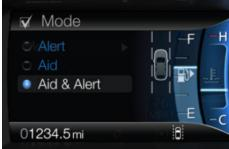
Lane assist is accessed in the lefthand cluster display using the left-hand five-way steering
