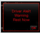
If the driver does not respond to this alert and the system continues to sense the driver is fatigued, another warning and chime will be issued. Drivers can monitor their condition on the dashboard at any time.
