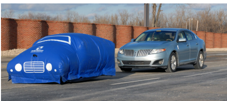
Adaptive cruise control and collision warning with brake support balloon-testing on Lincoln MKS.
