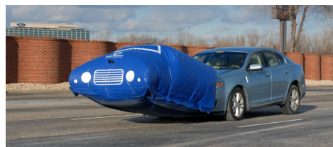
Adaptive cruise control and collision warning with brake support balloon-testing on Lincoln MKS.
