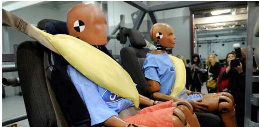
Ford inflatable safety belts combine the attributes of traditional safety belt and air bag technologies to help further reduce the risk of head, neck and chest injuries for rear-seat passengers.
