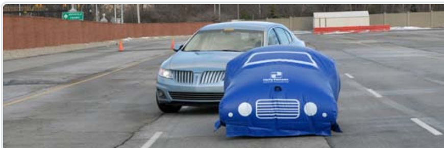
Ford is testing an array of active safety technologies by driving prototypes into large, car-shaped balloons.
