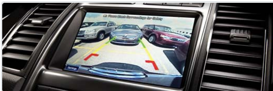
In the 2010 Ford Taurus, the rearview camera projects through the centerstack-mounted screen.
