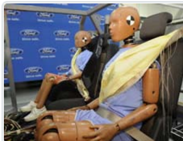
Ford introduces the auto industry's first-ever production inflatable seat belts, which are designed to provide additional protection for rear-seat occupants.
