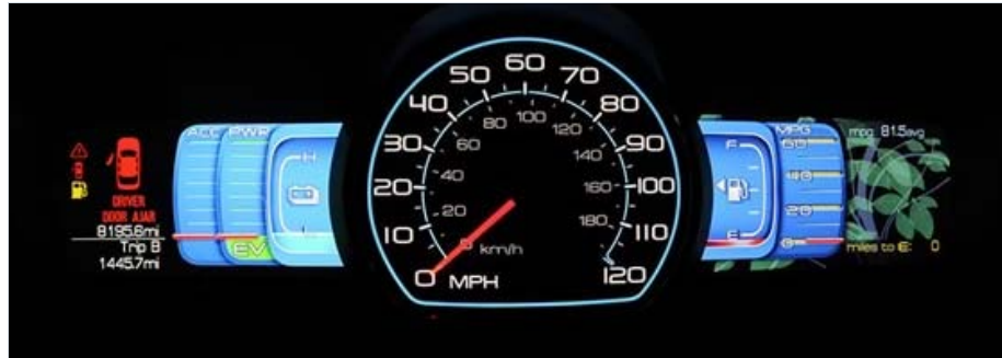
The Ford Fusion Hybrid's SmartGauge™ with EcoGuide gives drivers information to help them maximize fuel efficiency.
