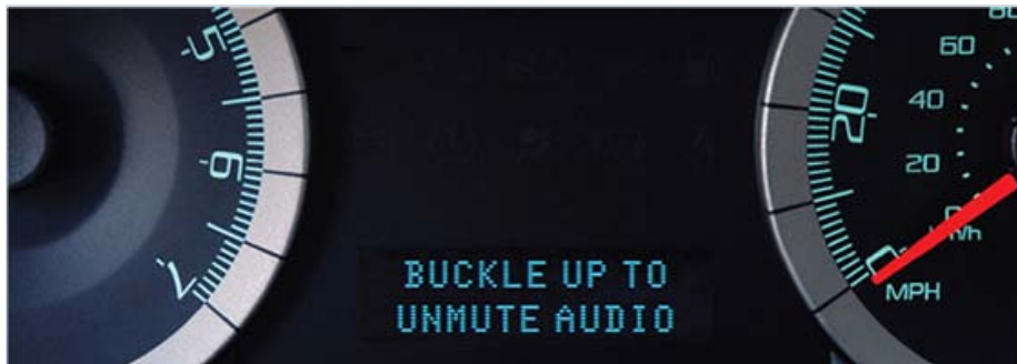
MyKey™ Insistent Beltminder™: If the MyKey driver and/or passenger does not buckle, then the vehicle will display a warning and mute the audio system.
