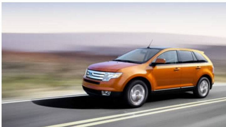
2007 Ford Edge CUV: With a 250-horsepower V-6 paired with a wide-ratio 6-speed automatic transmission, the 2007 Ford Edge delivers a projected 24 miles per gallon on the highway.
