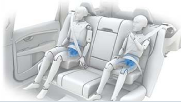
Integrated two-stage booster seat, which helps to protect children who have outgrown their toddler seat
