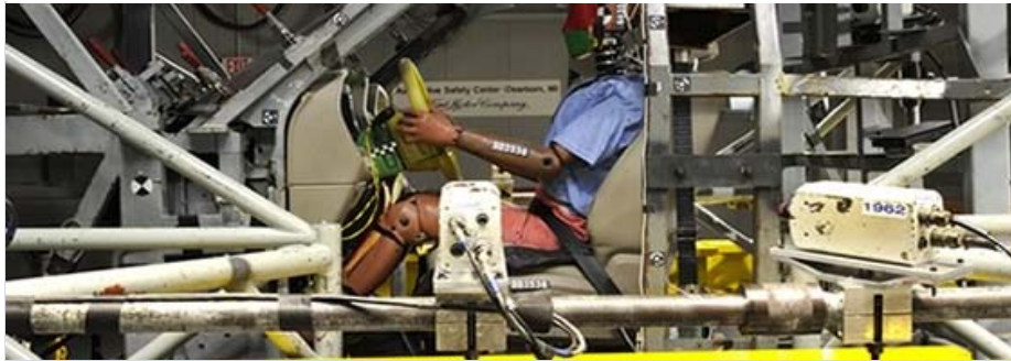
Servo-Hydraulic Reverse Crash Simulator, known as the Servo sled
