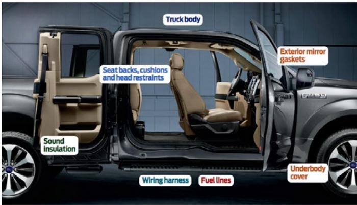
See the recycled and bio-based materials used on the new F-150.
