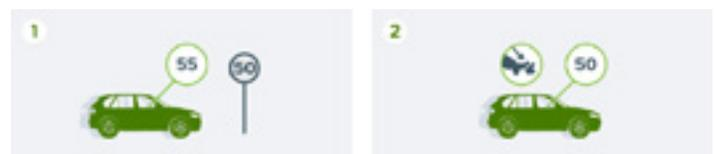
Combines ASLD with Traffic Sign Recognition to automatically adjust the set speed to the detected speed limit. Additionally, the driver can adjust the set speed manually and override the limitation (as described under ASLD, above).
