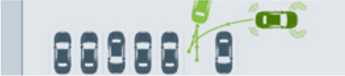
Active Park Assist, which helps drivers with parallel parking, is now available with enhancements including Perpendicular Park Assist (PPA) and Park Out Assist (POA), which helps drivers back into a perpendicular spot as well as exit a parallel parking space.
