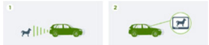
Transmits a rear-facing image when the driver selects reverse, making maneuvering while backing up or parallel parking safer and easier.
