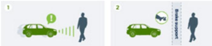
Uses a radar and a camera to scan the road and, if a collision risk with a vehicle or a pedestrian is detected, provides a warning to the driver. If the driver does not respond in time, the system can automatically apply up to full braking force to help reduce the severity of or even eliminate some frontal collisions.
