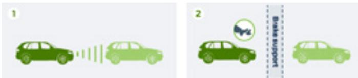
Ford Active City Stop helps to avoid or to mitigate accidents at low speeds. A LiDAR sensor detects objects in front of the vehicle and if it detects a collision risk with a vehicle, the brakes are precharged. If the driver does not respond in time, the system automatically applies the vehicle's brakes and reduces engine torque.
