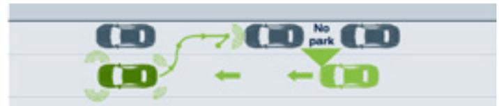
The system uses ultrasonic sensors to assess the viability of potential parallel parking spots. When a suitable space is found, Active Park Assist steers the car into the space while the driver controls the gears, accelerator and brake.
