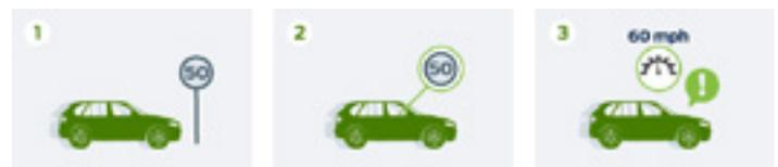
A camera recognizes speed limit signs; the driver is informed of the speed limit, and is also warned when that limit is exceeded. This technology currently recognizes signs that comply with the [Vienna Convention on Road Signs and Signals](#).
