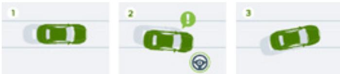
Using a forward-facing camera, the system warns the driver of unintentional lane departures. With Lane-Keeping Alert, the steering wheel vibrates when drivers stray from their lane, while Lane-Keeping Aid provides a mild steering input to encourage drivers to steer toward the center of the lane.
