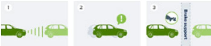
Uses radar, similar to ACC, to assess range and speed, and activates a visual and audible warning when the system detects a risk of collision with the vehicle in front. In addition, the brake system is precharged and brake assist sensitivity is increased to provide full responsiveness when the driver applies the brakes.
