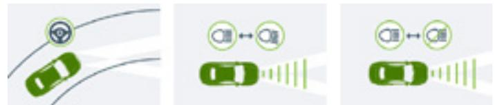
This includes semi-automatic high beam control, rainlamps and adaptive headlamps with beams that move in the same direction as the steering wheel and provide more visibility when driving around a curve.
