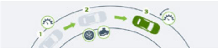
Assists the driver with maintaining control over the vehicle when entering a curve too quickly. It reduces engine torque and increases brake pressure to help keep the vehicle under control and follow the intended path. The technology is designed to be effective on wet or dry surfaces, and is expected to be helpful when drivers are entering or exiting freeway ramps too quickly.
