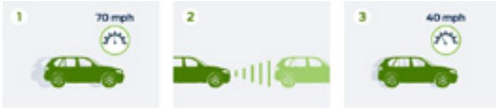
Helps drivers maintain a preset distance from the vehicle in front, using a radar that measures the gap and closing speed.
