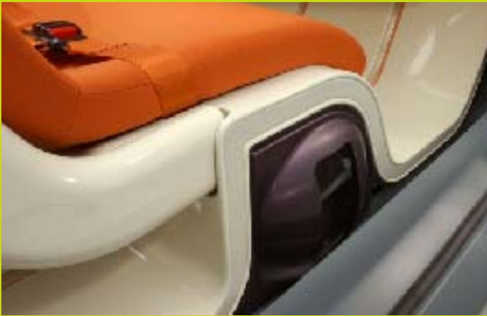
Hydrogen fuel tanks are located under the front and rear seats.
