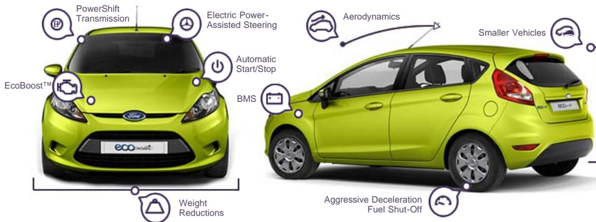
This section outlines our plans for improving the fuel economy of traditional gas and diesel engines. These actions include implementing advanced engine and transmission technologies, weight reductions and aerodynamic improvements, as well as increasing the efficiency of vehicle sub-systems.
