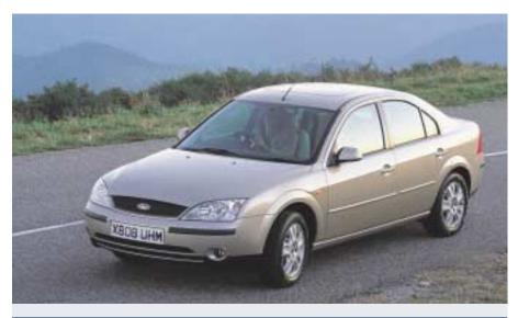
The 2001 Ford Mondeo, sold in Europe, contains 55 parts made of recycled, non-metallic material and 21 parts made of renewable material, (of which 10 parts also are recycled). This includes an air channel footwell made of recycled bottle caps, a fan and shroud radiator made of recycled carpets and an insert door trim panel made from kenaf natural fibers.
