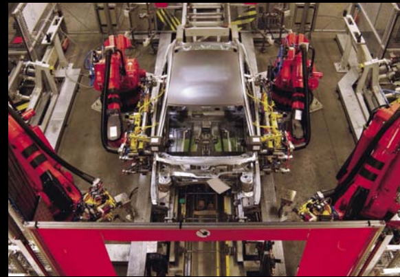
Robots weld the roofs of the new Volvo S40 and Volvo V50 at the Volvo Cars plant in Ghent, Belgium, where 5,300 employees work to ensure high vehicle quality.
