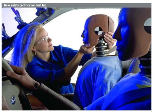
Cindy Bohen, Ford Safety Project Engineer, adjusts a dummy seated in a vehicle buck secured to Ford's new state-of-the-art Servo-Hydraulic Reverse Crash Simulator in Dearborn. The Servo sled accurately simulates full vehicle collisions by providing the same dynamics of a vehicle crash test without destroying the test device.
