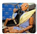
In 2010, Ford is bringing to market the world's first automotive inflatable seat belts, combining traditional seat belt and air bag technologies to help reduce head, neck and chest injuries for rear seat passengers.
