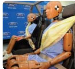
In 2010, Ford is bringing to market the world's first automotive inflatable seat belts, combining traditional seat belt and air bag technologies to help reduce head, neck and chest injuries for rear seat passengers.
